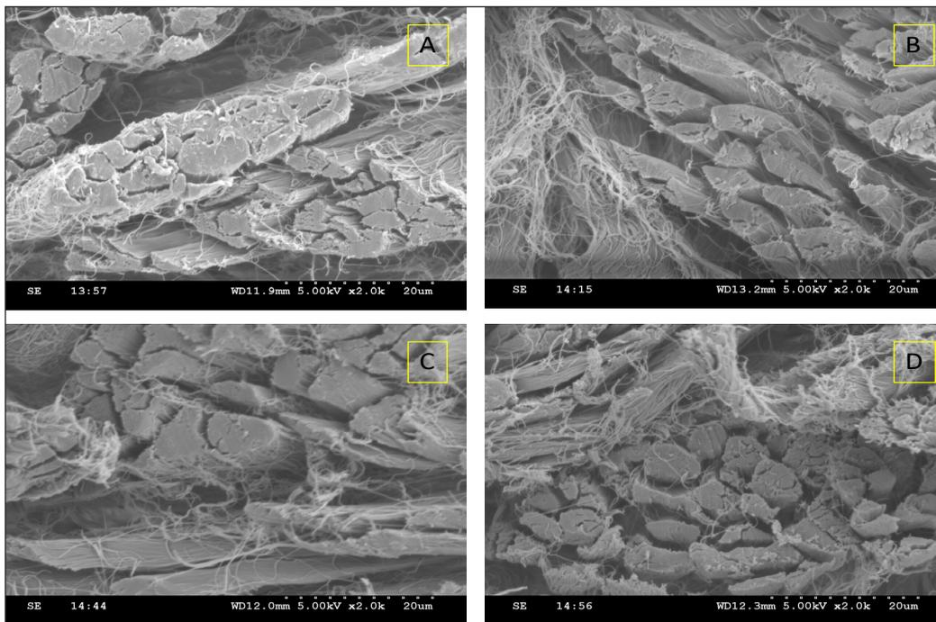
Figure 7. Scanning Electron Microscopy (X2000) of Chrome Tanned Goatskins Processed with: A-NC; B- PC; C- A1 (PURE); D- A2 (BLEND)
