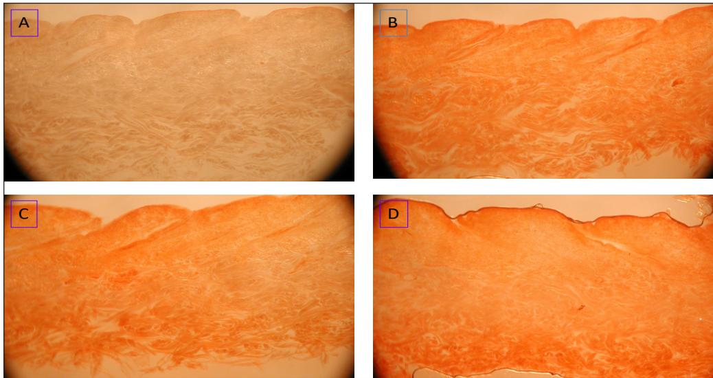
Figure 6. Staining Test Results Showing Cross-Section of Chrome Tanned Goatskins Processed with: A-NC; B- PC; C- A1 (PURE); D- A2 (BLEND)
